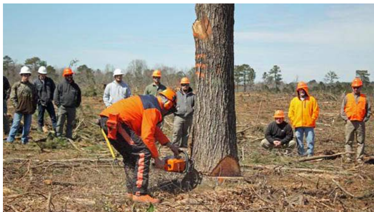
Bryan Wagner demonstrates the back-cut as part of his timber felling class.
