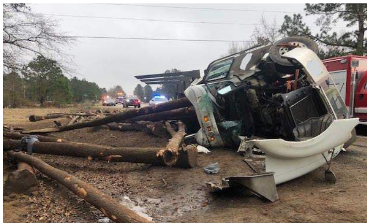
The result of a passenger vehicle pulling out in front of a log truck loaded with tree length hardwood pulpwood. Without a trailer mounted headache rack installed, the driver suffered life threatening injuries in his attempt to avoid hitting the passenger vehicle.
