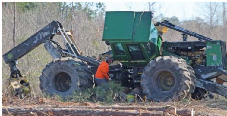
It is important to follow lock-out, tag-out procedures when servicing equipment.
